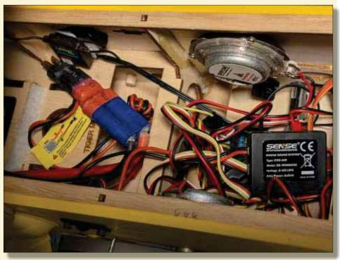
Top and bottom are the two speakers/transducers that are glued directly to the sides of the fuselage. In this case, the fuselage is balsa-skinned so the devices could be installed easily.
